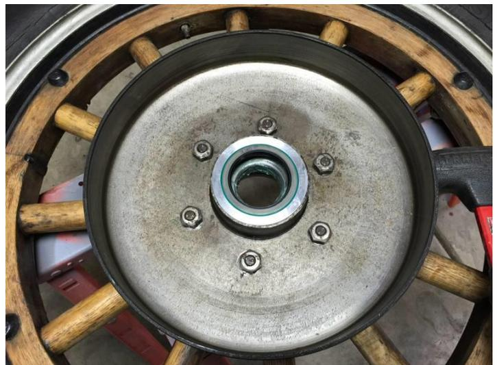
So step one repack the bearings with Marine grease while the adaptor gets cold. I'm not going to be able to pack them later. With the wheel on saw horses I tapped the adaptors into place and then the seals. I hope this is a permanent fix at least for my life time.
