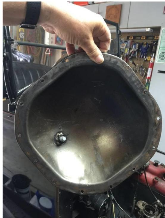
the rear end housing cover and found it clean no sludge but with a drain plug on the botto
